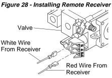
Figure 29 - Connecting Wires
